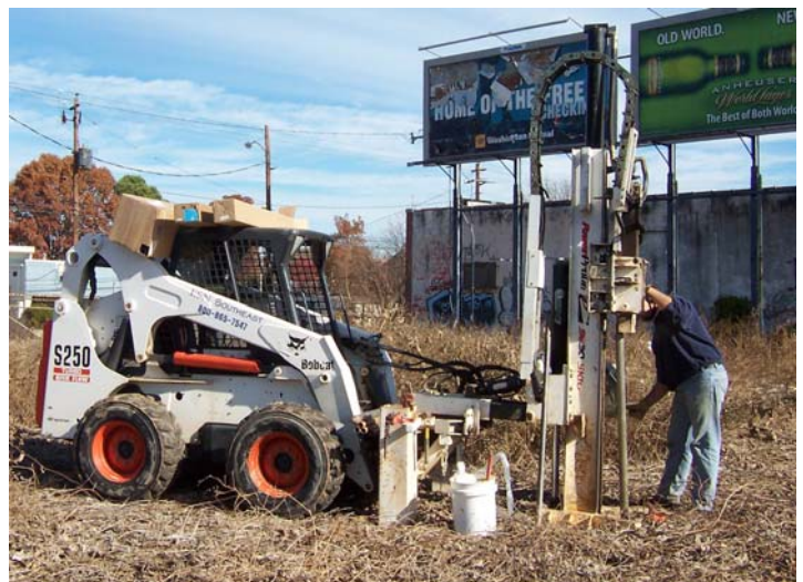
Use of DPT for rapid characterization at an AEM Brownfields site
